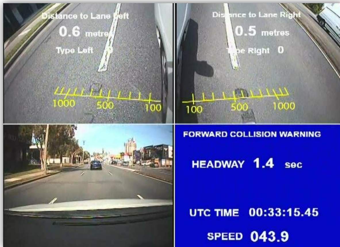
Sample screenshot outputs from VBOX showing headway and lane position
